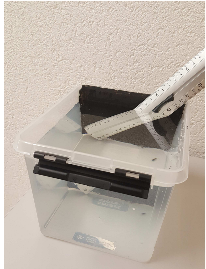
FIG. 15. A convenient setup for the ruler. It is best to fill water to the rim and to look into the water from above at a flat angle. Photo by Jean-Pierre Eckmann.
